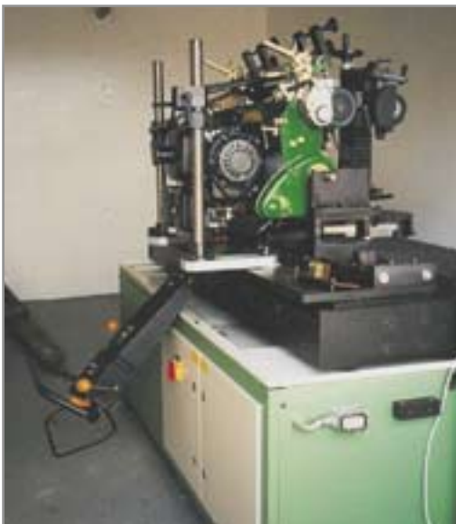
Manual putting-green mower clamped in position without needing to be dismantled
