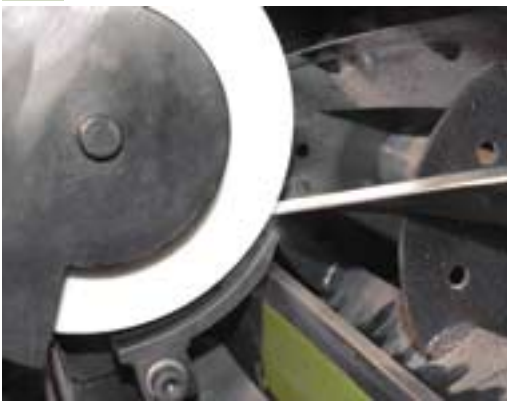
Grinding on the support pin
