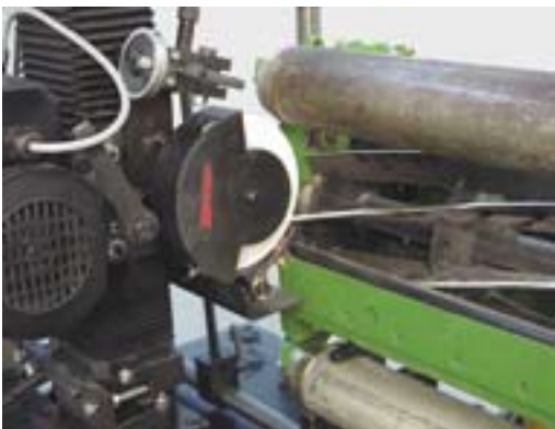
Sturdy bed-knife support promotes grinding operation
